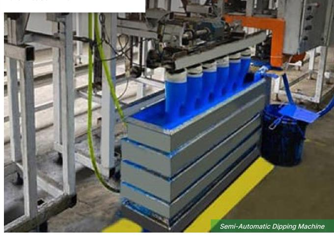
Duramitt Sdn Bhd, a manufacturer of various specialised protection gloves, has successfully transformed its dipping process by implementing a closed-loop inverter control system to enhance efficiency, reduce manpower, and improve product quality.
